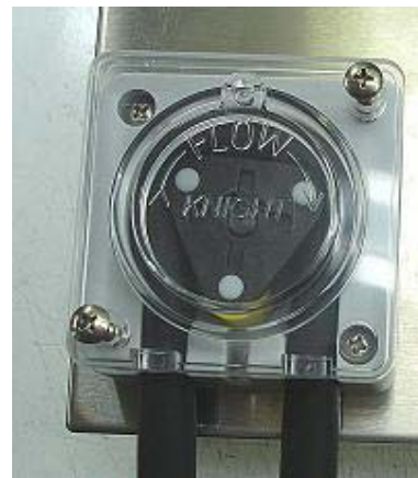
Figure 14. Top Cover replaced.
