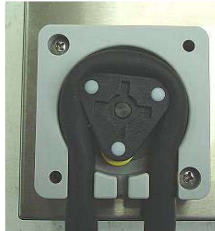
Figure 13. Rotor with new Tube fitted
