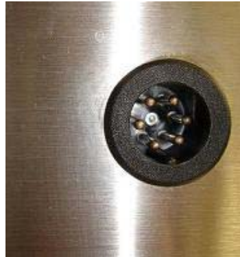
Figure 6. Controller connection socket
