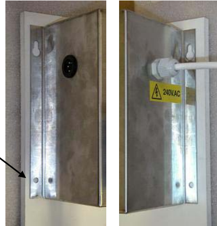
Figure 3. Peridoser Case Mounting Screw Location.
