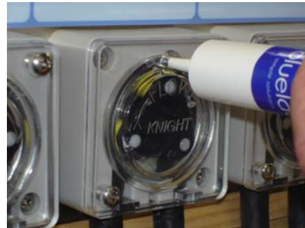
Figure 9. Peridoser Top Lubrication Point
